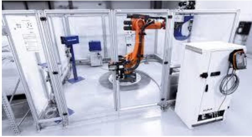
Traditional style of robot "locked" in a fenced compound
