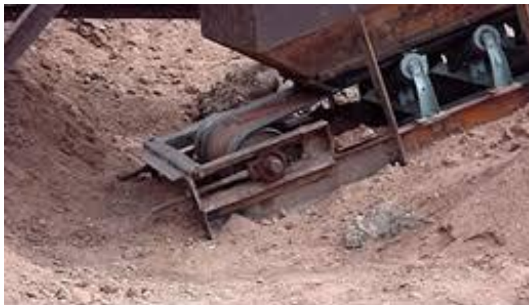
An unguarded conveyor
