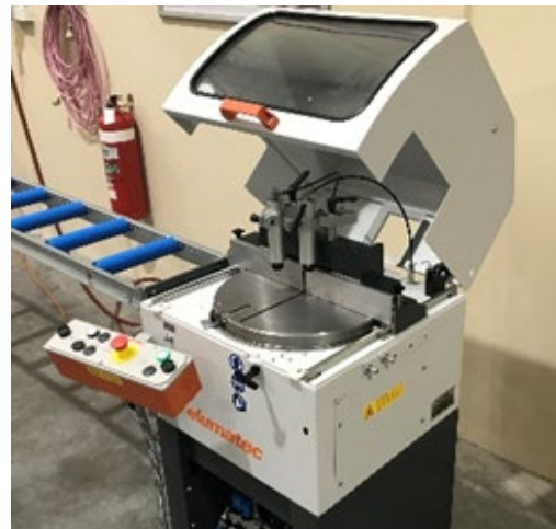
Modern saw with interlocked cover and normally retracted blade and 2-hand controls
