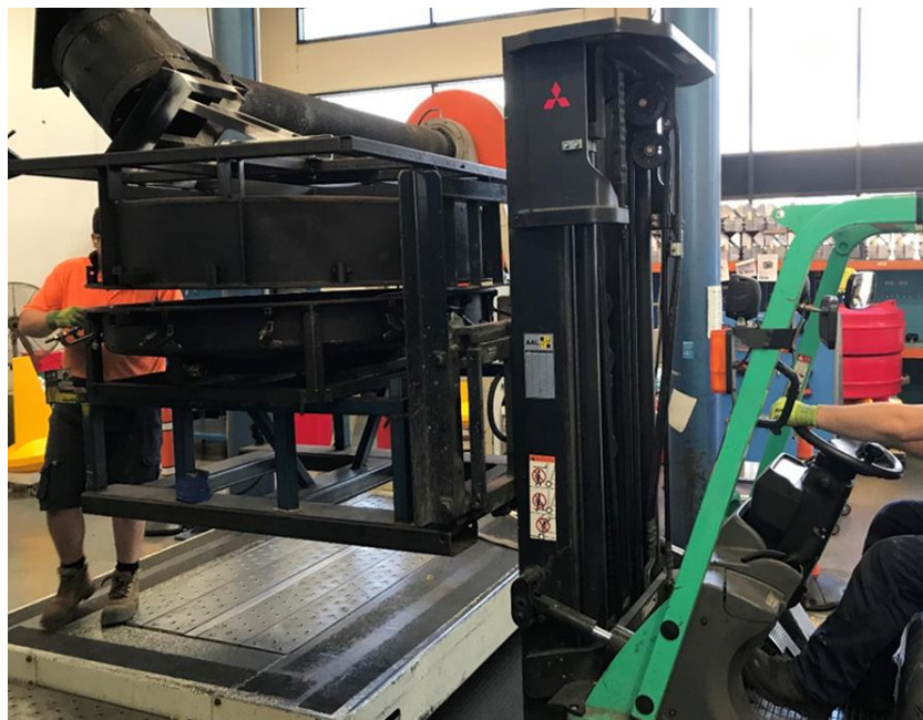
Worker unbolting a frame while held on forklift tines
