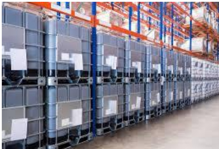
IBC storage 2-high in a racking system
