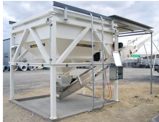
A fixed hopper and conveyor loader
