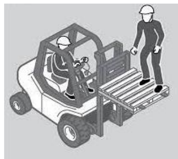
Examples of people standing on tines or pallet on tines – both dangerous and illegal
