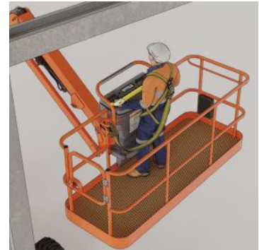
EWP near overhead steel beam
