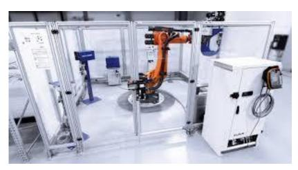
Traditional style of robot "locked" in a fenced compound
