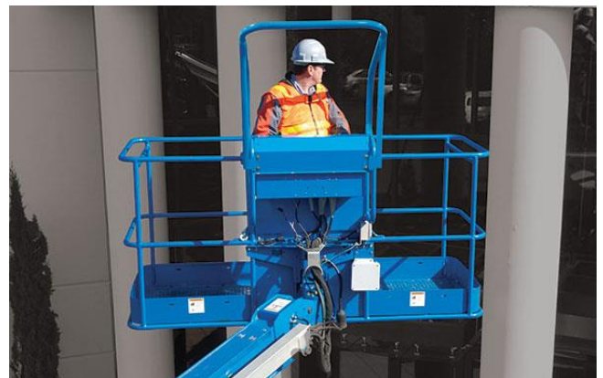
Boom lift with operator protective structure to prevent operator from being crushed against overhead obstructions. Image genielift.com.au
