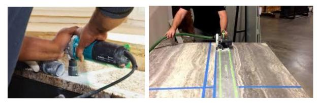
Cutting artificial stone benchtops Note: cutter on right has a dust extraction tube to minimise airborne silica dust in work area
